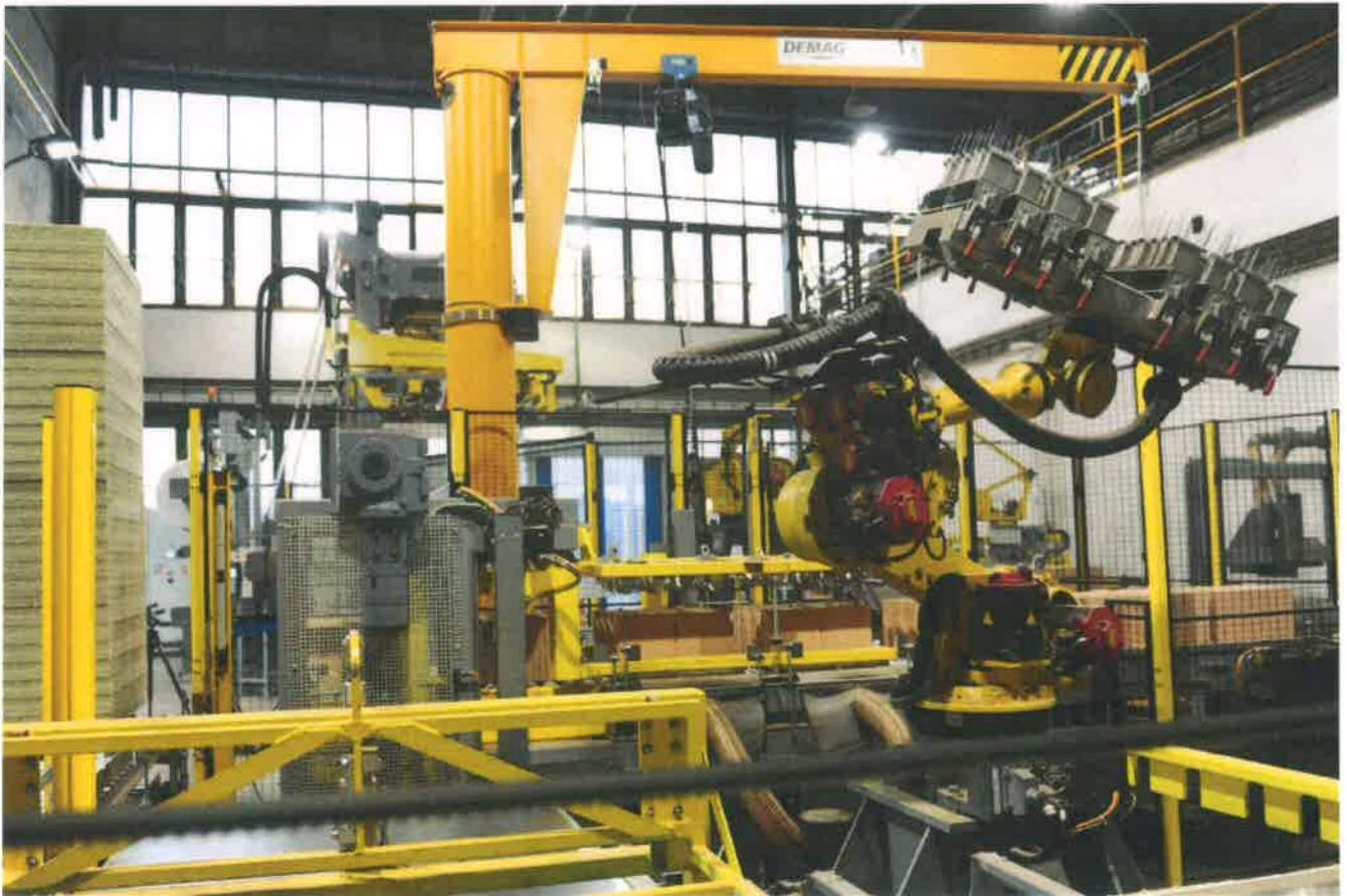
Photo 3 - Industrial robot for inserting thermal insulation pads into brick blocks
